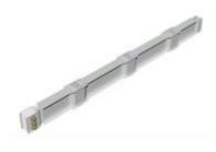
XCP-S - straight element for distribution (Cu).  $N^{\circ}$  of outlets 3+3 - Length 2.5-3m - In= 1600A
