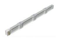
XCP-S - straight element for distribution (Al).  $N^{\circ}$  of outlets 3+3 - Length 3m - In= 1600A
