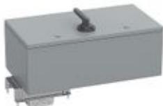
Tap-off box bolt on type (630A, Cu) with disconnector switch AC23 and fuse carrier base NH3 - In=1000A - IP55
