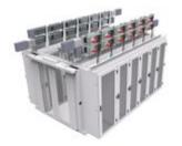
Data Center straight elements (IP40). Aluminium conductors and windows on both sides (2+2, step 800 mm) - In=315A - IP40 - length 1,6m
