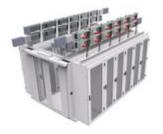
XCM linear element for data centers. Aluminium conductors and 4 windows per side (pitch 600mm) - In=1000A - IP40 - length 2.4m
