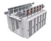
Data Center straight elements (IP40). Aluminium conductors and windows on both sides (4+4, step 600mm) - In=630A - IP40 - length 2,4m
