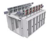
Data Center straight elements (IP40). Aluminium conductors and windows on both sides (2+2, step 600mm) - In=315A - IP40 length 1,2m
