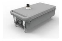
Fiber glass plastic tap-off box for MEGATIKER Mccb's installation (not supplied) - In= 250A - Type 3 - IP55 (cover with disconnection device)
