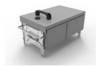
Metallic tap-off box with fuse-carrier for 3 fuses NH00 (fuses not included) - In= 160A - Type 1 - IP55 (cover with disconnection device)
