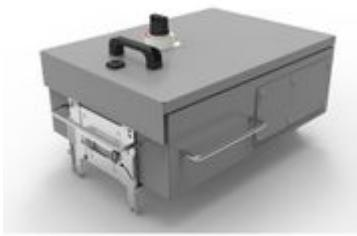
Metallic tap-off box for DRX3 HP MCCB's installation (not supplied) - In= 250A - Type 2 - IP55 (hinged cover with disconnection device)
