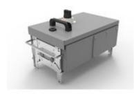
Metallic tap-off box for MEGATIKER MCCB's installation (not supplied) - In= 63/125/160A - Type 1 - IP55 (hinged cover with disconnection device)
