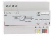
KNX modular power supply with RESET button and signaling LED for: -overload -Power supply -reset Bus connection via red black KNX connector. Input voltage: 120-230V at 50 ... 60 Hz. Output voltage: 29V + 2 / -1V d.c. SELV. Auxiliary output voltage 29V + 2 / 0V d.c. SELV. Output current: 640 mA. Installation on DIN rail, dimensions 7 DIN modules
