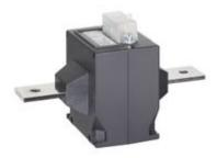
TAQ20P - Current transformer, single-phase for protection - Cable/passing bar: winding primary - Ratio: 300/5A - Class: 5P5/5P10 - Accuracy: 8/4VA
