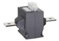
TAQ20P - Current transformer, single-phase for protection - Cable/passing bar: winding primary - Ratio: 60/5A - Class: 5P5/5P10 - Accuracy: 8/4VA
