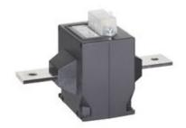
TAQ20P - Current transformer, single-phase for protection - Cable/passing bar: winding primary - Ratio: 30/5A - Class: 5P5/5P10 - Accuracy: 8/4VA
