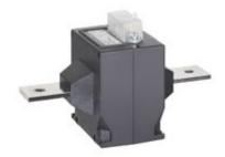
TAQ20P - Current transformer, single-phase for protection - Cable/passing bar: winding primary - Ratio: 10/5A - Class: 5P5/5P10 - Accuracy: 8/4VA
