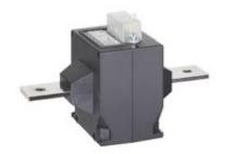
TAQ20P - Current transformer, single-phase for protection - Cable/passing bar: winding primary - Ratio: 250/1A - Class: 5P5/5P10 - Accuracy: 8/4VA
