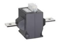
TAQ20P - Current transformer, single-phase for protection - Cable/passing bar: winding primary - Ratio: 60/1A - Class: 5P5/5P10 - Accuracy: 8/4VA
