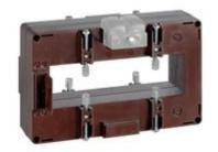
TAS127 - Current transformer, single-phase - Cable/passing bar: 38x127mm - Ratio: 500/5A - Class: 0.5/1 - Accuracy: 2/4VA
