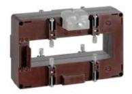
TAS127 - Current transformer, single-phase - Cable/passing bar: 38x127mm - Ratio: 750/1A - Class: 0.5/1 - Accuracy: 4/8 VA
