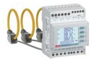
Kit Nemo D4-Le + 3 current sensors Rogowski ø 190mm -Multifunction for application in LV - Network: single-phase or three-phase 3/4-wires unbalanced - Display: LCD backlit -Dimension: 4 DIN modules - Output: none - Current: 5A - by CT dedicated 5÷8000A (41 primary selectable range) - Output: pulse S0 / 1 alarm contact + RS485 BACnet - Input: 80÷500Vac - Auxiliary supply: 80÷265Vac or 100÷300Vdc
