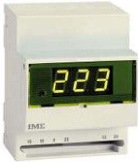
DGM D4 - Digital voltmeter/ammeter current (input by CT) or voltmeter AC RMS (direct input) 1000 points - Dimension: 4 DIN modules - Input: 1A or 500V - Aux: 115Vac - Viewing: 5÷8000A (38 selectable range)/direct 500 V
