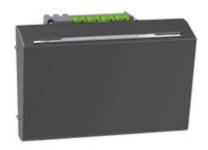
Badge-holder pocket for the power supply inside the hotel room - slot light with built-in lamp - 30 second switch-off delay - max. load 30 VA Power supply 230 V a.c. - 3 modules - dark
