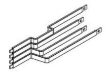
Connection kit for M1 160 and external busbar compartment for with busbars 800A in aluminium - section 20x5mm
