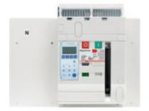
Fixed version air circuit breaker 4P - In= 2000A - Ue= 690Vac -Icu= 100kA - Frame 2
