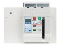
Fixed version air circuit breaker 4P - In= 4000A - Ue= 690Vac -Icu= 50kA - Frame 2
