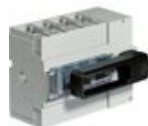
T7234WF/160 Disconnector MW250 - 4P - 160A - 690Vac...
