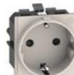
KM4141A German standard socket 2 P+E 16 A 250 V ...
