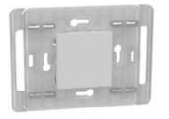
Wireless light switch No-Battery. It allows the ON / OFF and dimming control of one or more connected devices for the lighting control. Surface installation with repositionable stickers (supplied) or onto a flush mounting box without any wiring - can be combined with the 3-module cover plate item JA4819... or, if the ends of the support are removed, with the 2-module plate item JA4802... - 2 modules - White
