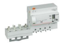
Earth leakage module with measure function integrated 4P - type A-HPI - In= 125A - Vn= 400 Vac - time setting (0-0,3-1-3s) and current setting (0,03-0,3-1-3A)
