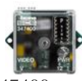
347400 Interface for the conversion of the coax...
