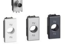
Terminal coaxial socket, -10dB attenuation, for centralised TV systems, also remote powered, and centralised satellite systems with current and signal transfer for channels selection; shielded connection clamps with captive screws - Ø 9,5 mm - male connector - incorporated impedance final adapter 75 ? - supplied in package with common mechanism and front covers in different aesthetic finishes - 1 module
